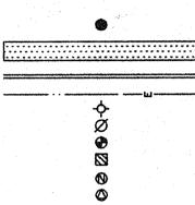
Property Monument Concrete Concrete Curb Overhead Electric Hydrant Power Pole Gate Valve Catchbasin Sanitary Manhole Gas Meter
