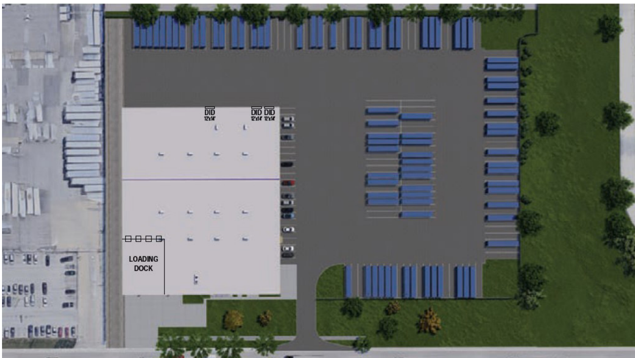
TRAILER PARKING CONCEPTUAL RENDERING 140 STALLS @ 10' 53' 70' DRIVE AISLES
